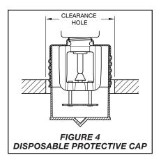
Step 6. After the ceiling has been completed with the 2-1/2 inch (63,5 mm) diameter clearance hole and in preparation for installing the Cover Plate Assembly, remove and discard the Protective Cap, and verify that the Deflector moves up and down freely. If the Sprinkler has been damaged and the Deflector does not move up and down freely, replace the entire Sprinkler assembly. Do not attempt to modify or repair a damaged sprinkler.
